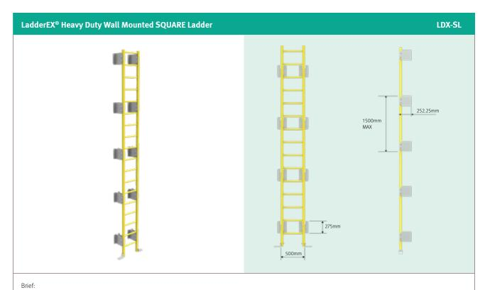
For industrial and other heavy duty purposes, Treadwell supplies a more durable and robust heavy duty wall mount and floor mounts (if required) for that added safety
